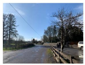
Location 14 - Left Hand Bend On L3402 Direction Continue At This location Visual inspection indicates that rear projection of blade will oversail third party land on offside to avoid telegraph pole on nearside.
